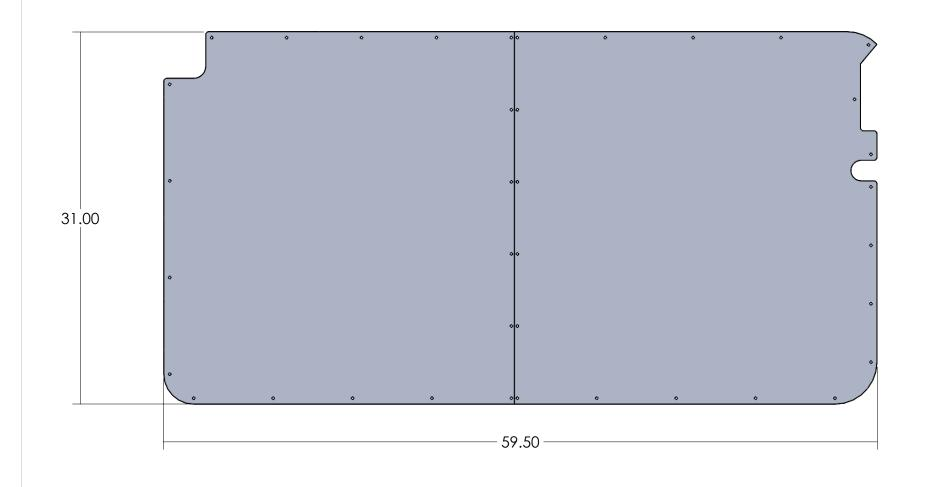
Description 13+ RAM ProMaster Lo-Roof Door Panel - Rear Full - Driver - Solid Rev. Weight Material Item No. 050131 17.55 Lbs. Aluminum 642002 #8 x 3/4" Phillips Washer Head Tek Screw PROPRIETARY AND CONFIDENTIAL SIZE Date 642366 3/16 x 1/4 Grip - Alum-Steel Dome Head Rivet - Open End TRUPRIEMATION CONTINUED IN THIS
