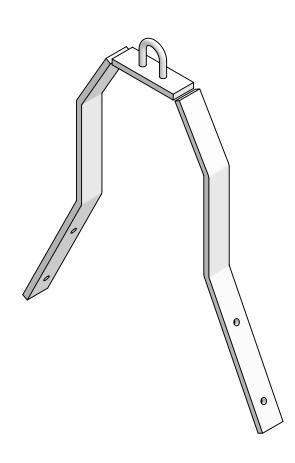
Note: Requires drilling 3/8" diam. holes for mounting (2 holes on each side).
