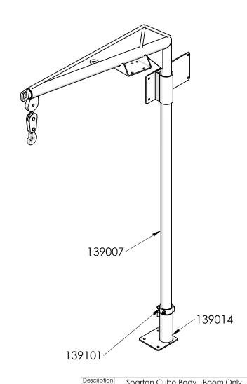
Spartan Cube Body - Boom Only -Rear Driver/Passenger Rev. Weight Material Steel 130131 50.37 Lbs. PROPRIETARY AND CONFIDENTIAL SIZE Date THE INFORMATION CONTAINED IN THIS DRAWING IS THE SOLE PROPERTY OF JAM TRILCK SODIES. ANY REPRODUCTION IN PART OR AS A WHOLE WITHOUT THE WRITTEN PERMISSION OF J&M TRUCK BODIES IS PROHIBITED. 5/3/2021 Drawn By. S.Gutierrez SCALE: 1:18 7541 Chapman Ave Unit B Garden Grove, Ca 92841
