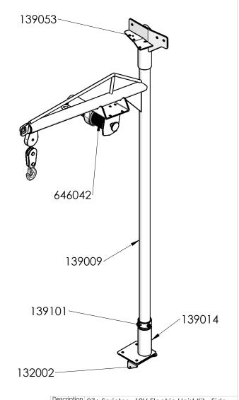
Description 07+ Sprinter - 12V Electric Hoist Kit - Side Door B-Pillar - Passenger Side Material 130047
