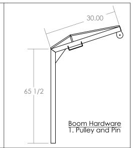
1) First place the Upper Mount onto the Boom followed by the Lower Mount. After both mounts are on the boom stand the Boom and the Upper Mount into place on either the Driver or Passenger side of the door jam - depending on your hoist set up - hold the Upper Mount properly in place and measure the Upper Mount so that the bottom of the mounting tube is 51-1/2" from the floor. Clamp the Upper mount into place.
