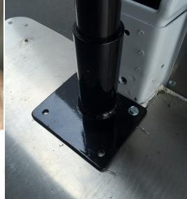
It is recommended to double check that the hoist column is square to the van using a large square. If needed adjust the Lower Mount position. (Please do not use a level to do this because the van does not sit level and will not make the boom square to the van.)
