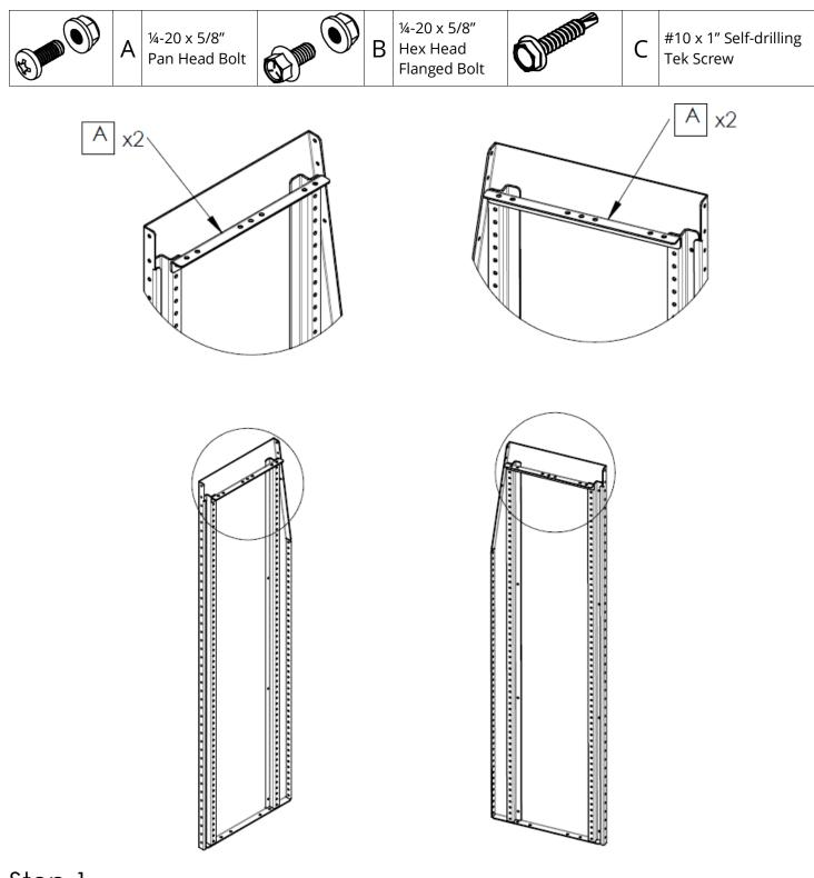
• Bolt one L-bracket to each end panel Note: L-brackets must be flush to the top of the rails
