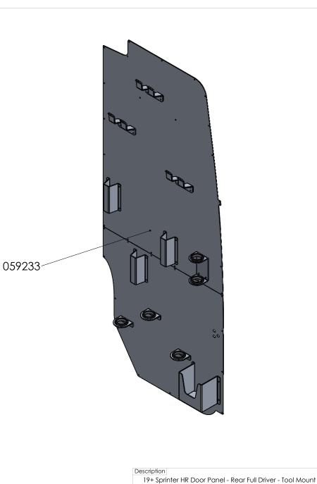
Rev. Weight Material Item No. 050233 20.70393 Lbs. ---Aluminum PROPRIETARY AND CONFIDENTIAL SIZE Date THE INFORMATION CONTAINED IN THIS DRAWING IS THE SOLE PROPERTY OF JAM TRUCK BODIES, ANY REPRODUCTION IN PART OR AS A WHOLE WITHOUT THE WRITTEN PERMASSION OF J&M TRUCK BODIES IS PROHIBITED. 5/30/2024 Drawn By. S.Gutierrez 7541 Chapman Ave Unit B Garden Grove, Ca 92841 SCALE: 1:12 2
